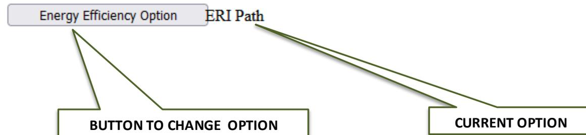
At the start of a new project or whenever the Energy Efficiency Option is selected, a new screen appears to set the energy option as described by IECC 2021 section R408
